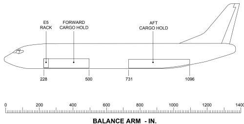
The following table provides cargo compartment locations, usable volumes and the corresponding volumetric centroid arms for cargo compartments with an E5 rack installed.
