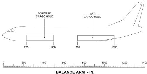
The following table provides cargo compartment locations, usable volumes and the corresponding volumetric centroid arms.
