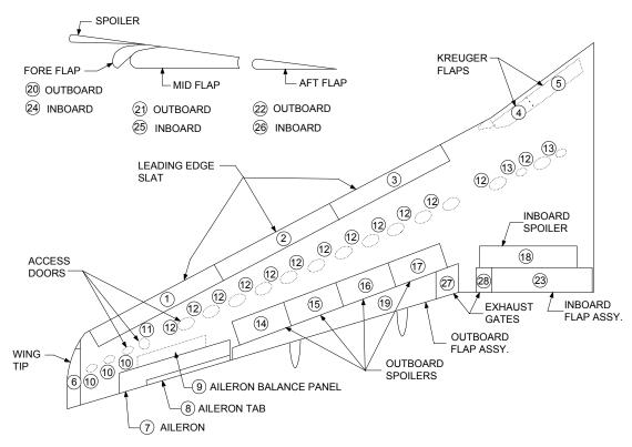
The following table provides nominal weights and balance arms for wing components from the above illustration. Values from this table should only be used to determine approximate weight and balance for specialized types of maintenance.
