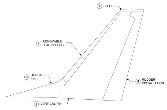
The following table provides nominal weights and balance arms for vertical fin components from the above illustration. Values from this table should only be used to determine approximate weight and balance for specialized types of maintenance.
