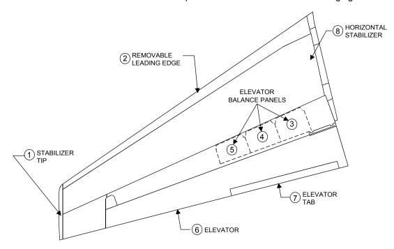
The following table provides nominal weights and balance arms for horizontal stabilizer components from the above illustration. Values from this table should only be used to determine approximate weight and balance for specialized types of maintenance.
