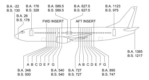
The following table provides Body Station to Balance Arm conversion data.
